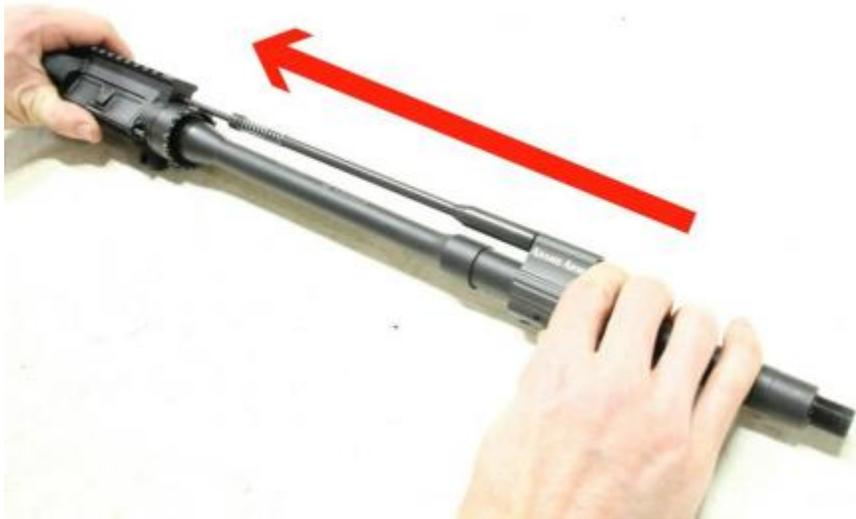
8. Position the gas block so it sits between .026 - .035 off the shoulder of the barrel. Using two business cards to space the gap. This will give you a good starting point for setting the correct gap.
