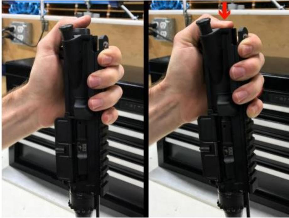
11. While you continue to hold the bolt carrier group in battery, use your free hand to move the drive rod up and down, ensuring that there is a gap between the drive rod and carrier.
