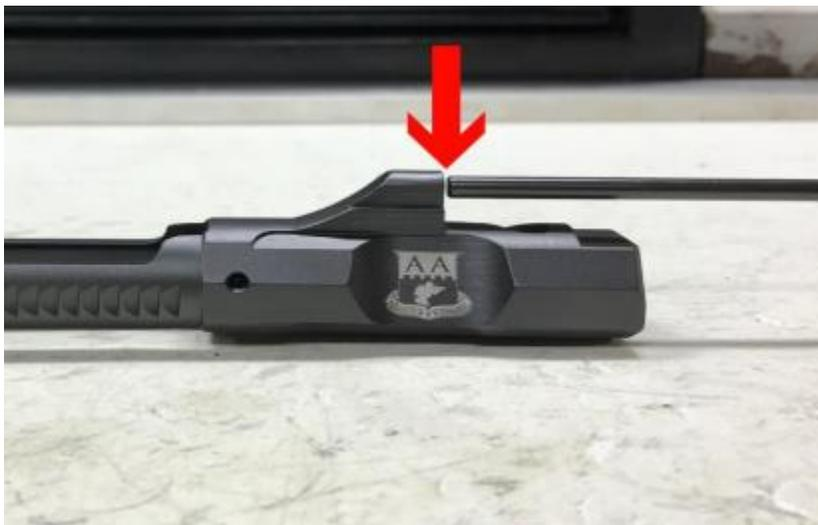
The spec for this gap is .015 - .025 inches. This gap has multiple important functional purposes. It allows for a slight amount of heat growth in the drive rod.
