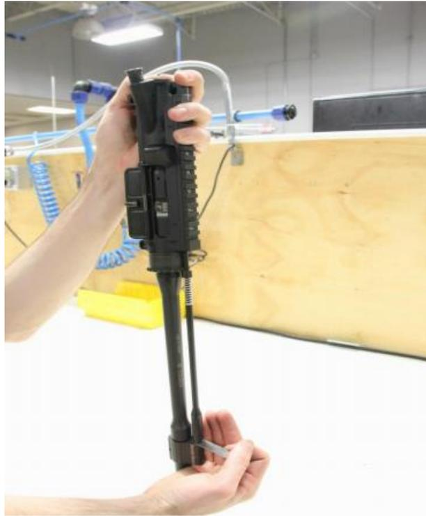
If the gap is larger than .025, use light hammer taps on the face of the gas block, to move the gas block backwards and close the gap. If the gap is less than .015, use light hammer taps on the back of the gas block to move it forward and increase the gap size. After making adjustments, re-measure with the gapping tool. Repeat process as necessary until the gap is correct.
