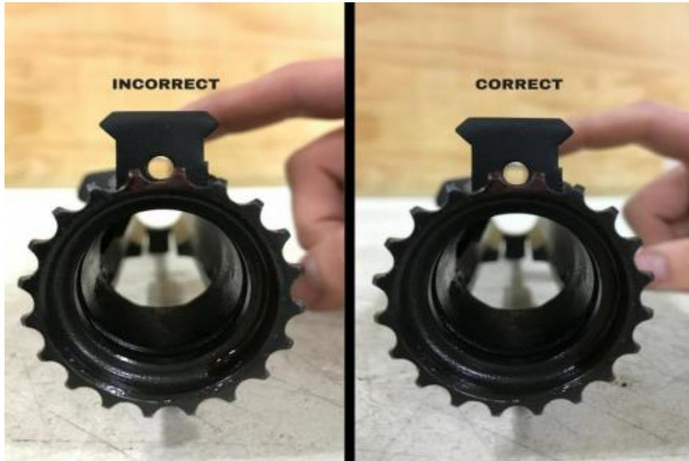
2. Use the drive rod to make sure that the barrel nut notch and receiver opening are properly aligned, by placing the striking end of the drive rod into the upper receiver opening, through the notch in the barrel nut. The middle of the drive rod cup should be perfectly centered with the gas port in the barrel.
