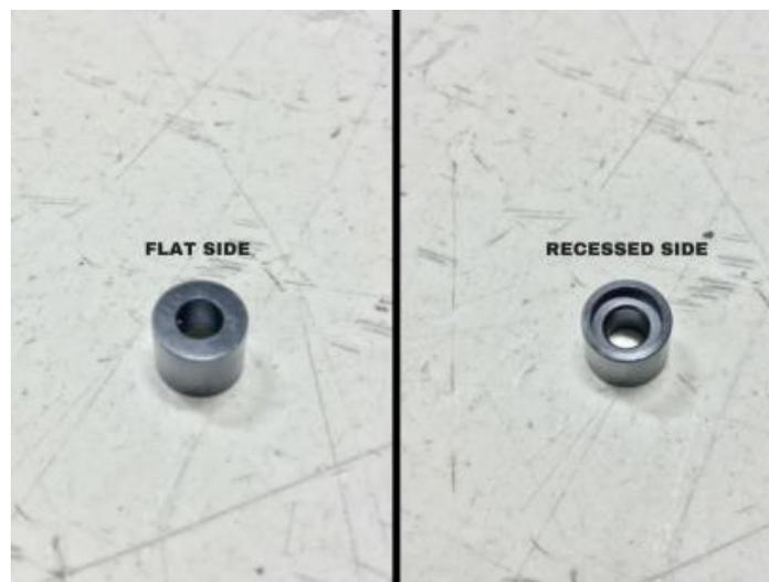
4. Slide the recessed side onto the striking end of the drive rod. Once it has reached the spring, push down on the bushing and twist, compressing the spring and locking the bushing and spring together
