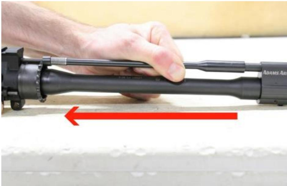
Note – some drive rods may not be perfectly straight, which can result in failing the binding test. However in these cases, you should be able to rotate the drive rod to find a free spot where it will drop correctly. As long as there is a position in the 360 degrees which a drive rod can rotate, that allows the drive rod to drop freely, it is passable.
