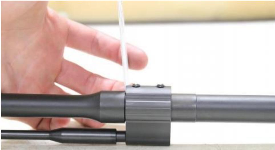
9. With the upper assembly laying on the table, and gas block positioned, put slight downward pressure on the barrel while holding the gas block in position. Tighten one of the set screws, enough to hold the block in place, but not enough to prevent you from repositioning the block with light hammer taps.
