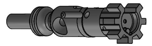
BOLT WITH EXTRACTOR REMOVED NOTE: Only separate the extractor spring from the extractor when replacement is necessary
