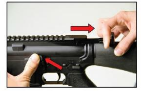
**3.** To lock bolt open, pull charging handle rearward, press bottom of bolt catch, and allow bolt to move forward until it engages bolt catch. Return charging handle forward.
