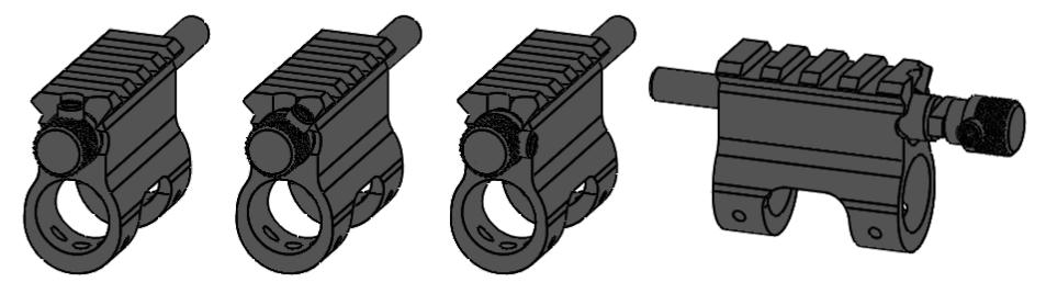
The 12 o'clock or "High" position opens the gas plug completely, allowing the firearm to use the total amount of gas pressure. With this position, you may fire semi-automatic as the rifle was originally designed to. If the firearm is functioning correctly, you will be expelling empty casings between the 2 and 4 O'clock position (roughly around the right shoulder) from the receiver consistently.
